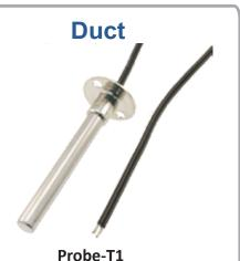
The Probe-T1 is a certified Pelican 10K temperature probe for detecting air temperature in a closed duct system. The flat end of the probe is able to seal against a metal surface to reduce air leakage. Common applications for this probe would be supply or return air temperature monitoring.
