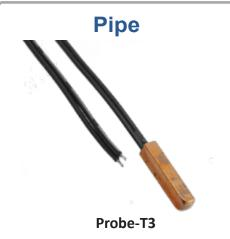
The Probe-T3 is a certified Pelican 10K temperature probe for detecting the temperature of a pipe or metal surface. The probe is housed in copper allowing for accurate temperature conductivity. Common applications for this probe would be detecting boiler or chiller pipe temperatures.
