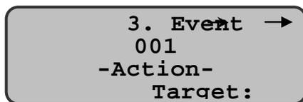
Actions are comprised of two parameters. **TARGET** identifies the component that will perform the action. The following three components may be programmed:
