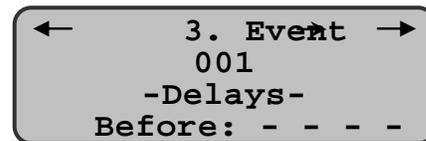
The **BEFORE** and **AFTER** delays may be programmed at 30 seconds, 45 seconds, or from 1 to 99 minutes by increments of 1 minute. The five dashes (- - - -) indicate that no delay had been programmed. The **AFTER** delay can also be put into latch mode.
