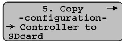
This section of the COPY MENU is only accessible if an SDcard is present. Data can be transferred from the controller to the SDcard, or from the SDcard to the controller. Thus, an image of the controller's programming may be transferred and stored on a computer. Similarly, the controller's programming may be executed on a computer and then transferred to the controller.
