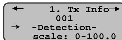
The DETECTION MENU does not appear for an Manning AirAlert™96d-RM8 relay module or Manning AirAlert™96d-AP annunciator panel.
