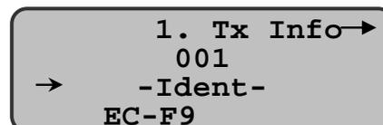
The identification of the network component is comprised of two parameters: the sensor name and the sensor type. A pre-programmed list of sensors is available for both.
