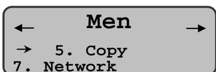
The cursor to the left of a field on the display indicates that this field is accessible. The arrows in the upper left and right corners indicate that a window is accessible at the left and right of the active window respectively. The keypad's four arrows serve to move the pointer in the MAIN MENU, and the *Enter* key is used to access the selected field.
