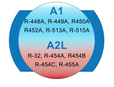
State and Federal regulations are now in place to phase down/phase out the use of high GWP HFC refrigerants. These regulations will impact new systems, on going service and retrofits. This class will introduce you to the next generation of A1 - A2L & Natural Refrigerants and their adoption in AC, Heat Pumps, Chillers, and Refrigeration.
