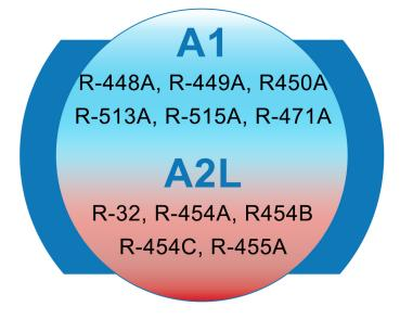
State an Federal regulations are now in place to phase down/phase out the use of high GWP HFC refrigerants. These regulations will impact new systems, on going service and retrofits. This class will introduce you to the next generation of A1 - A2L & Natural Refrigerants and their adoption in AC, Heat Pumps, Chillers and Refrigeration.
